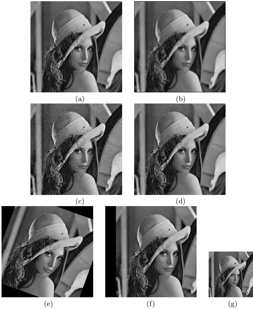
Fig. 4. ICs marked with cross: (a) original image; (b) 3 \times 3 average filtered; (c) 5(d) JPEG compressed image with compression ratio of 70; (e) 20 degree clockwise rotation of image plus cropping; (f) 30 pixels translated image along x axis; (g) scaled image based on scaling factor of 0.5
